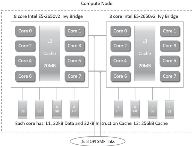
**FIGURE 1.** Illustration of compute node architecture with dual sockets, showing the physical cores within each socket, on-chip cache, and memory channels.
