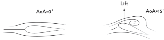
Fig. 1. The swirling around the front, or leading edge, of the wing is a result of the vacuum created above the wing, and is tied to the occurrence of the leading-edge vortices that play a dominant role in the occurrence and study of aerodynamic lift and stability in birds and commercial aircraft.
