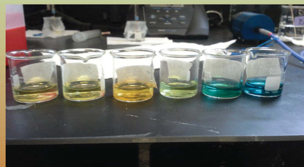
Figure 2. Time and concentration dependent coloration. From left to right: 0.02, 0.1, 0.5, 1.5, 10 mg/L of NH_4^+ with appropriate ratio of reagent 1 and 2 after 1-2 hours.
