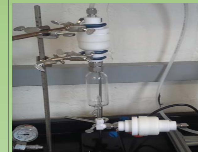
Figure 6. Left: Mist chamber set up used to create liquid sample from air 3 . Bottom left: syringe pump to be used to fill and empty mist chamber with liquid. Bottom right: reagent mixing system.
