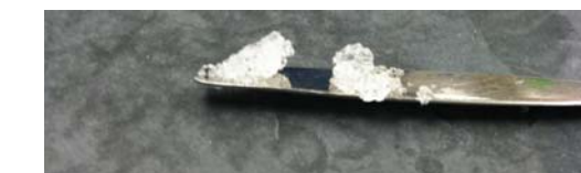
Figure 10. Transparent gellan beads before QBP was immobilized on their surface
